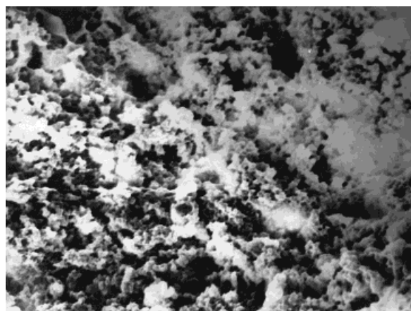
Figure 2 Porous poly(MAA-co-3G) obtained from dispersion polymerization (magnification \times 187.50 ).
